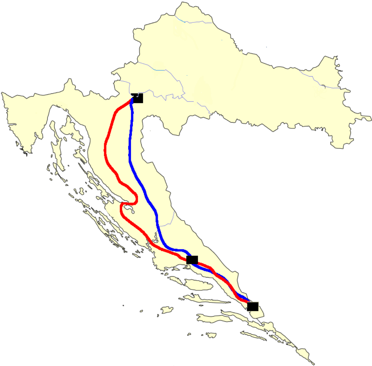
Figure 2: Approximate map of the actual A1 highway (in red) and the least-cost path (in blue). The black dots represent the nodal cities of Karlovac (in the north), Split, and Metković (in the south).
